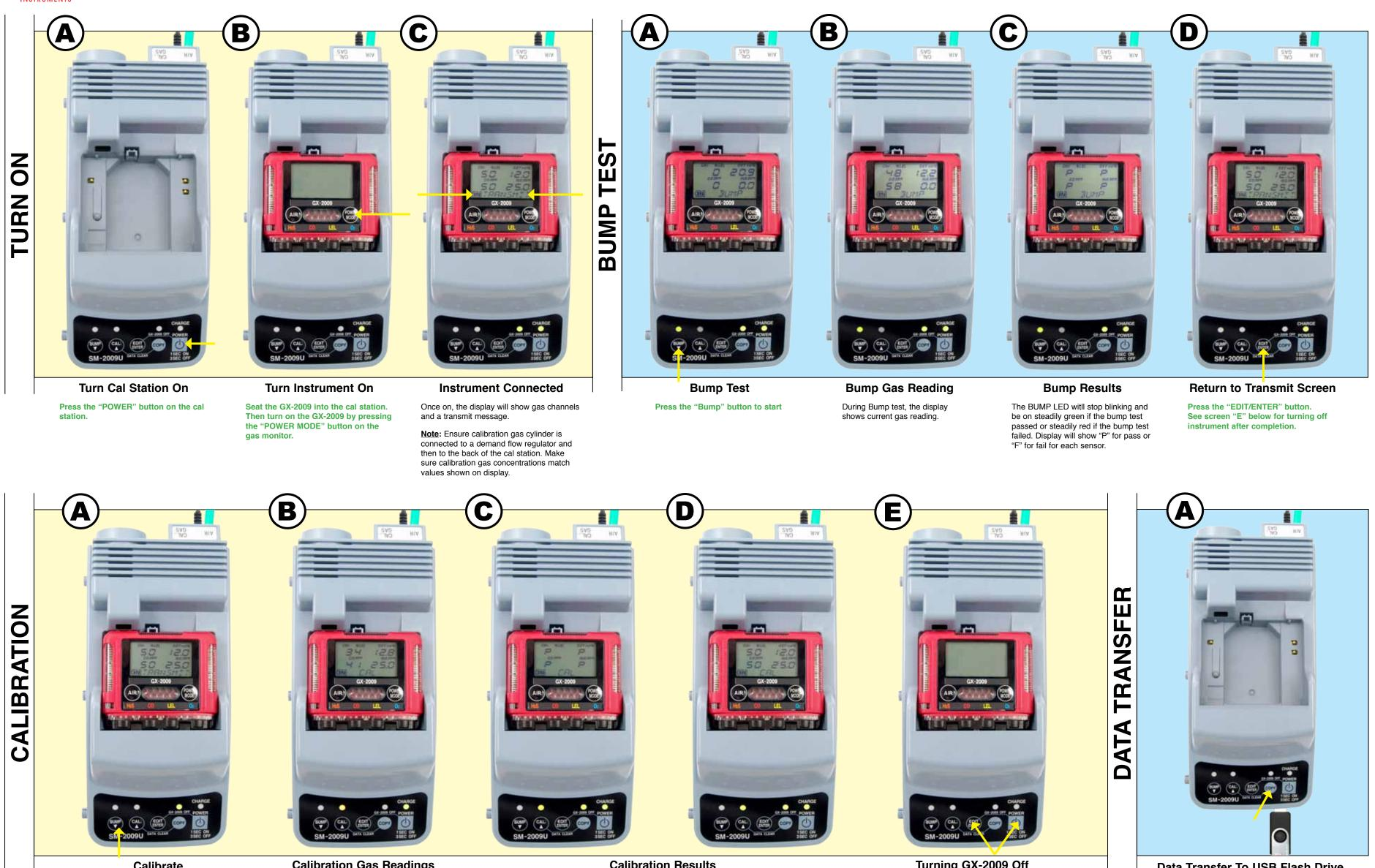
Calibrate Press the "CAL" button to start calibration.
